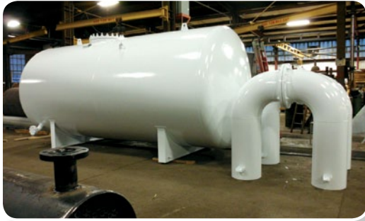
84" O.D x 160" OAL High pressure oxygen tank
