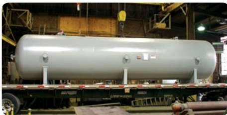
120" O.D x 420" OAL Low pressure oxygen tank
