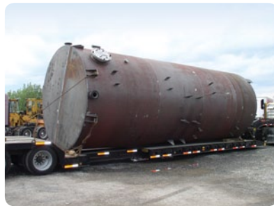
144" O.D X 420" OAL Housing Tank
