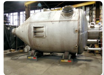
96" O.D x 214" OAL Vapor Chamber
