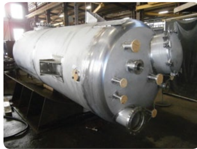
60" O.D x 240" OAL Process vessel
